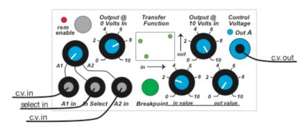
Note that the low resolution display provides a rough but useful indication of the transfer function. The actual voltages are calculated to a high degree of precision, and are appropriate for application to pitch and other variables.
