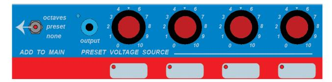
Only one "preset voltage source" can be selected at a time as indicated by the LEDs. The knob above each pad sets the output CV from 0-10v. The corresponding voltage will appear at the blue "output" banana when that knob/source is selected.
