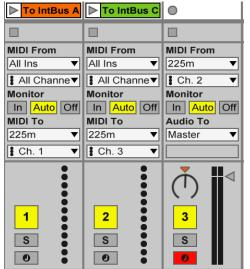
The example to the left shows the card being used to send Ableton MIDI clips to the Internal MIDI bus A and C as well as recording Internal MIDI bus B.
