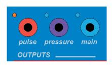
The **pulse** output is red banana on the upper left. A red LED will indicate every pulse output. The **pressure CV** output correlates to the detected amount of finger contact on the keys. The blue LEDs next to the pressure output will get brighter as the voltage gets higher.
