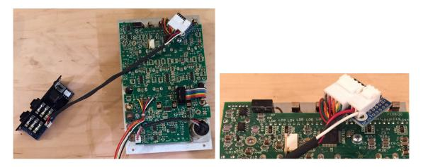
For use with a 207e or 206e, you replace the 5pin audio output cable with this little board as pictured. Restore the audio to the panel by inserting the 207e or 206e audio cable back in to the right angle 5pin header and then insert a 3pin cable into the 3pin header and plug the other end into the 22X-I-O.
