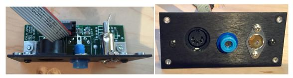
This can be combined with an old 225e I/O board with the unused MIDI out jack is removed and the USB position is nibbled to make room for the antenna mount
