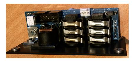
If the jumper was in the "St" [Stereo] position (connecting pins 3 and 4) then the left audio jack becomes a Stereo output.
