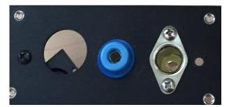
The 22X-I-O panel can be used for the 272e by using a washer or nut on the 12v banana connection and drilling small mounting holes for the antenna connector
