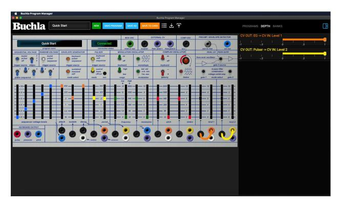
Connections are listed, color matched to their correlating banana cable, labeled with the output and input connections. Adjust the slider to the desired effect. Note: when inverting signals, you may need to adjust the correlating parameter's offset slider to put in the expected range.
