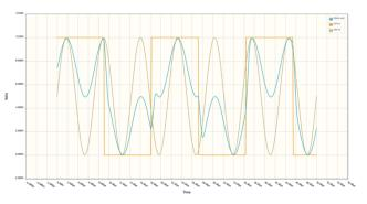
But when inverted the center reference for the inversion still influences/offsets the mix that then gets clipped at around 0v. This is because the inverted signal will mix before the 0v protection *In these examples, the orange line is the A input; the brown line is the B-input and the blue line is the output.*
